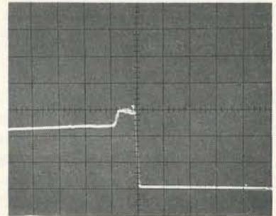
Fig. 11. A step down usually means an impedance mismatch, but the mismatch shown here is a problem of extreme proportions: using the wrong impedance cable! In this test of a computer-network cable, using the wrong type of cable results in garbled data that the interface card cannot read.
