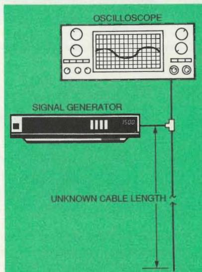
*Fig. 1. This setup will let you easily measure the length of a cable without using a tape measure. Connect a signal generator to one end of the cable and measure the amount of time it takes to see the steps in the waveform on an oscilloscope.*
